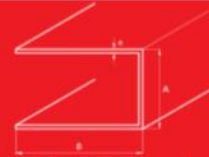
Perfigal Canal Perimetral
